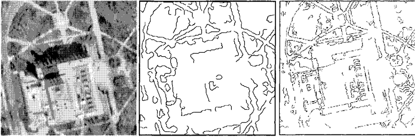
Figure 3. A section of a digital image showing the test site (left), the matched edges at 2-meter (center), and 1-meter (right) resolution.
